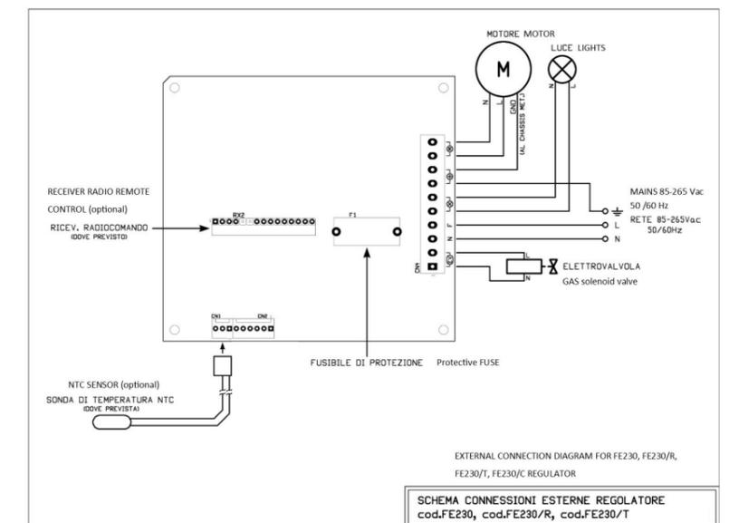
Fig.2: External connection diagram.
